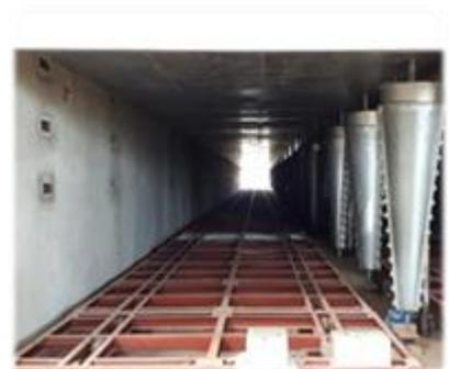
Figure 5 Tunnel drier and recirculation units
