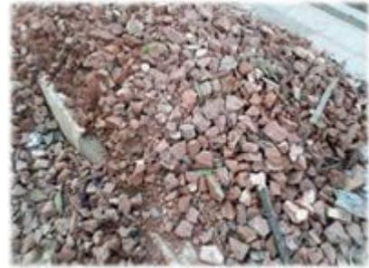
Figure 7 Stone produced from crushed brick
