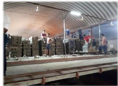
Figure 1 Manual offloading packing of kiln cars
