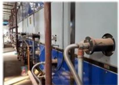
Figure 6 Gas fired side burners
