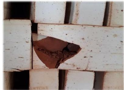
Figure 2 Product damaged during firing due to excessive moisture remaining after drying
