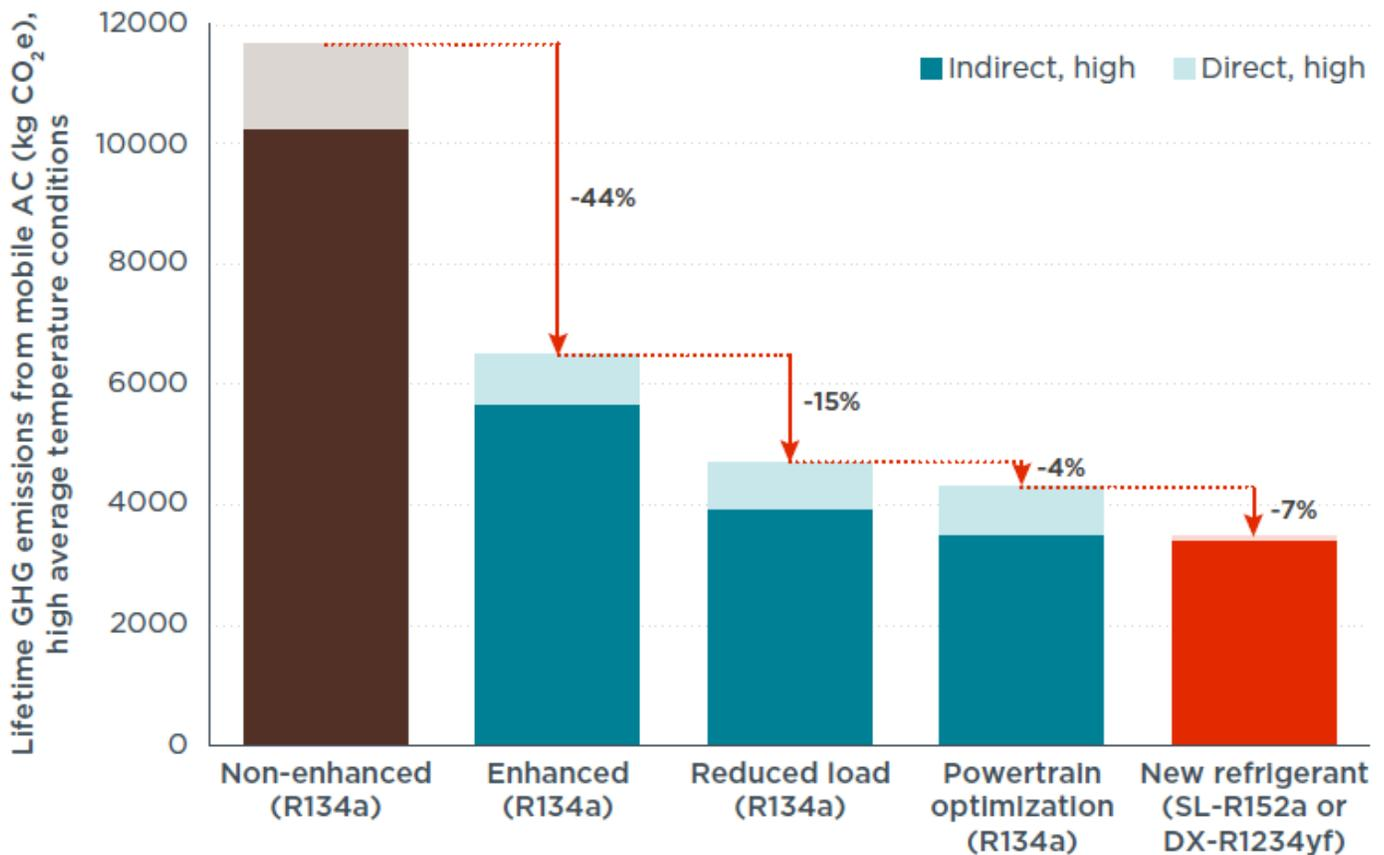
Figure 3: GHG reduction potential of improved MACs in climates with higher ambient temperature (Blumberg et al, 2019)
