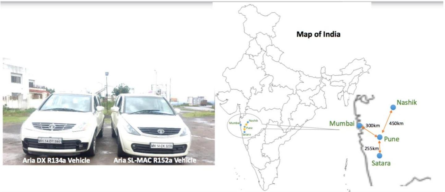
Figure 2: The baseline and SL-MAC R152a road-test vehicles and the test route in India.
