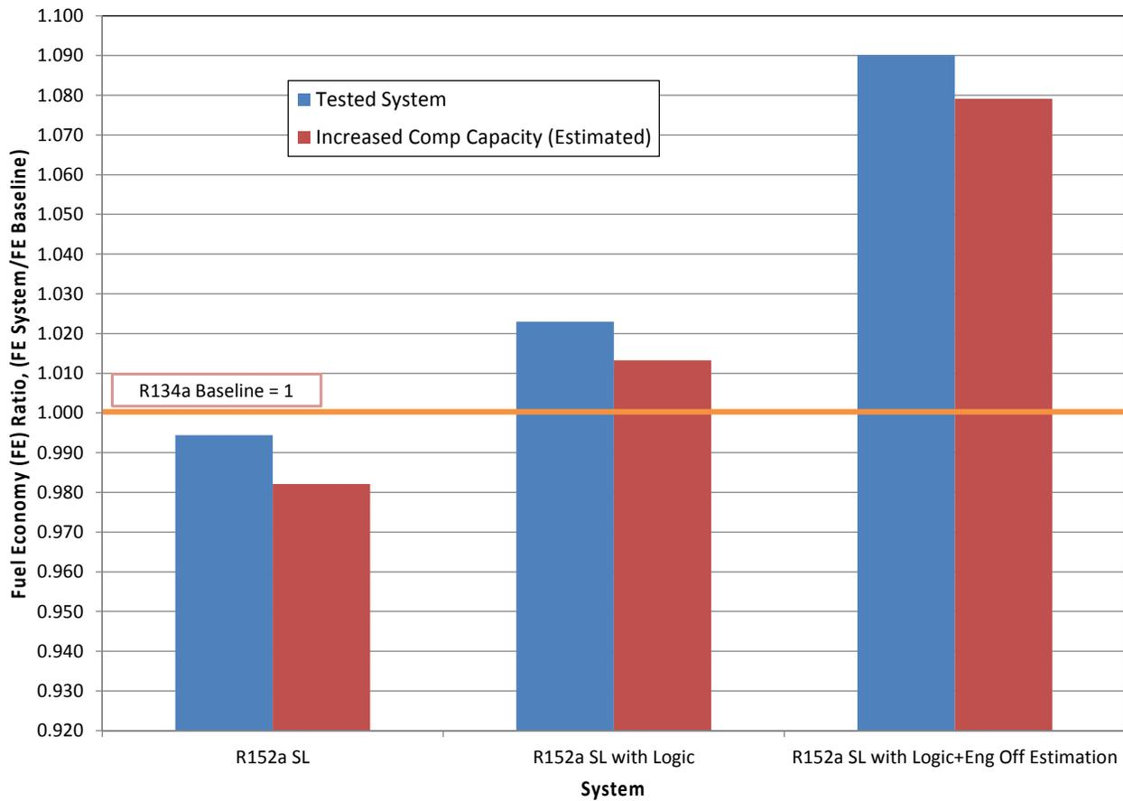
Figure 4: Estimated fuel economy impacts of increased compressor capacity and integration with stop-start (engine off) enabled vehicle.
