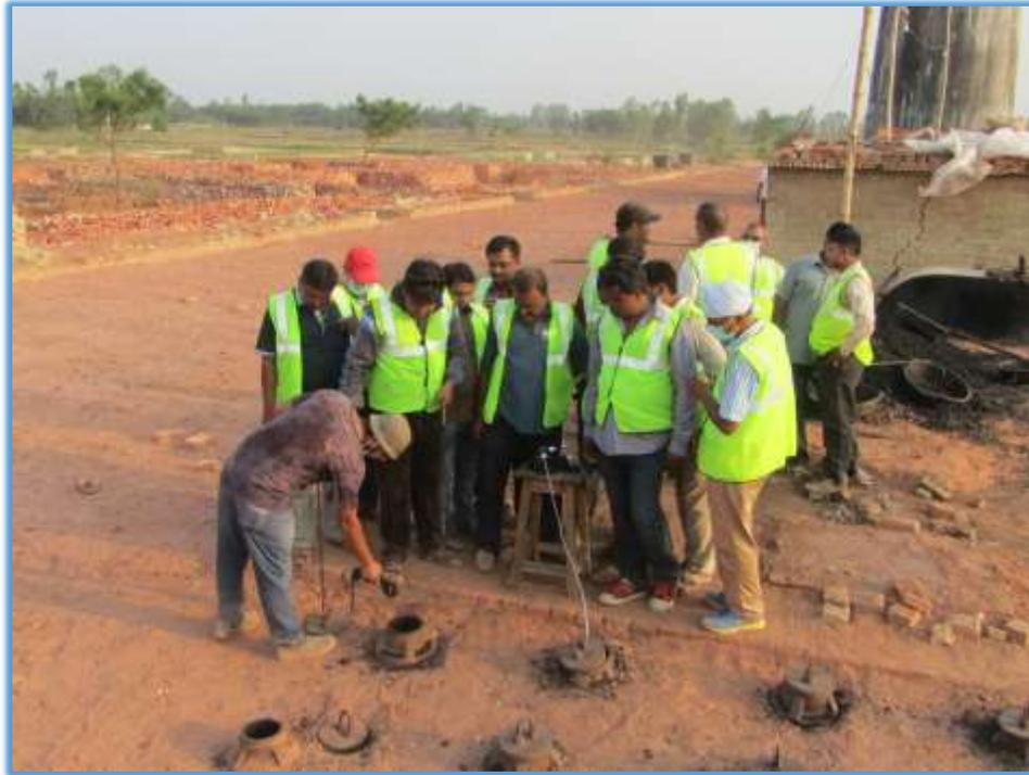
Photograph 5: Temperature measurement of firing zone
